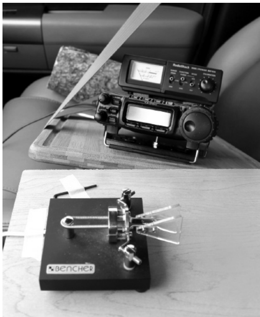
FIGURE 6-4 The W1GV mobile CW installation, showing the radio and SWR meter in the background and the keyer paddle in the foreground.
