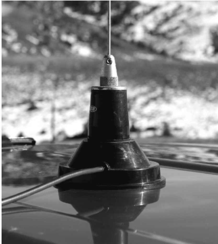
FIGURE 6-3 A magnetic base mount (also called a “mag mount”) for a VHF mobile ham radio antenna.
