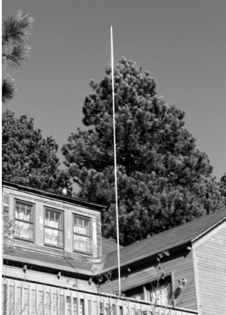
FIGURE 1-2 Here's a photo of the antenna for the ham radio station shown in Fig. 1-1 . It's made of telescoping sections of aluminum tubing, mounted on a deck railing, and can go up or come down in a couple of minutes to accommodate the rapidly changing weather conditions characteristic of my location.
