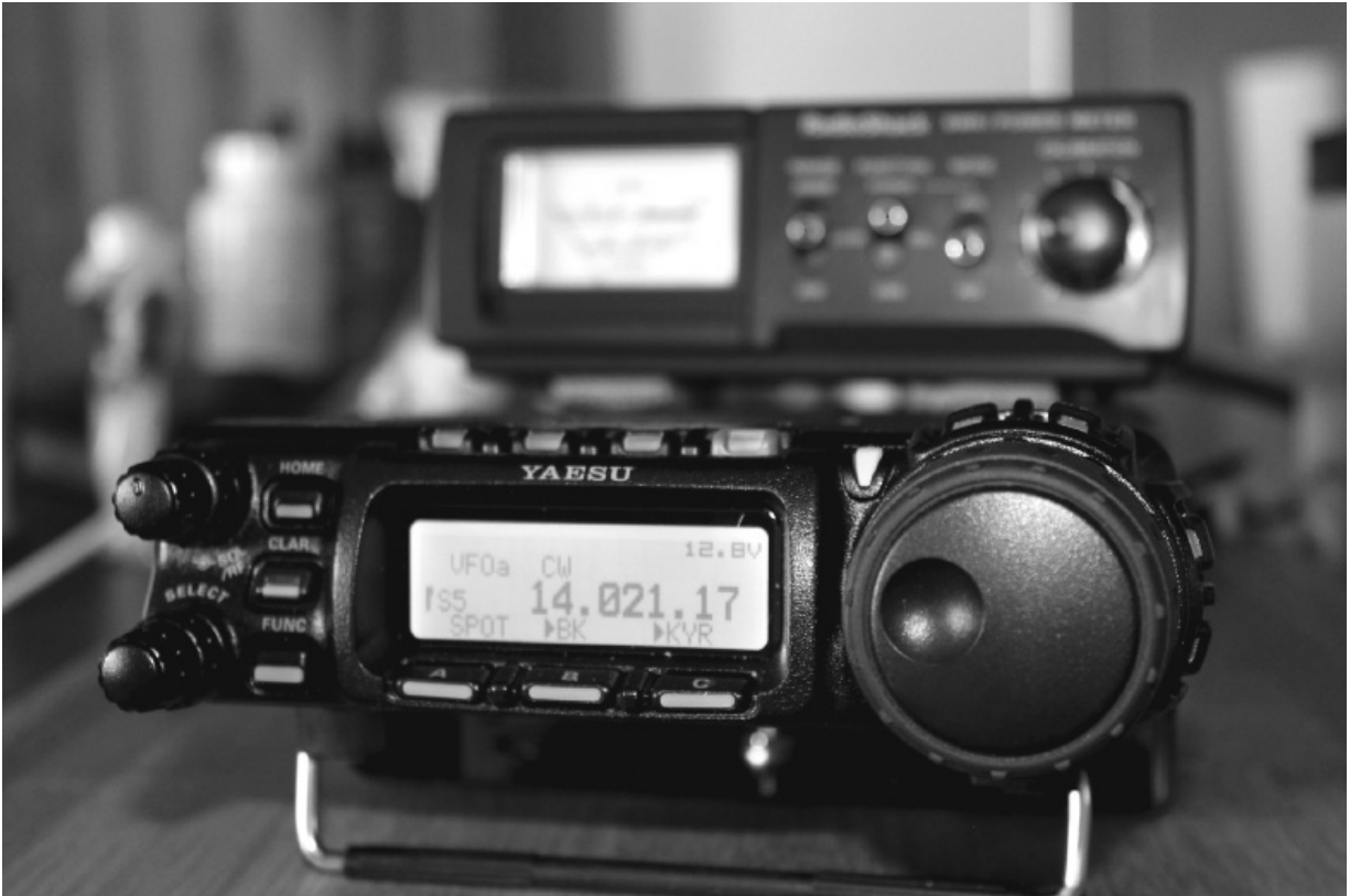
FIGURE 6-1 A mobile/portable ham radio transceiver that covers 160 meters through 70 centimeters in all popular modes.
