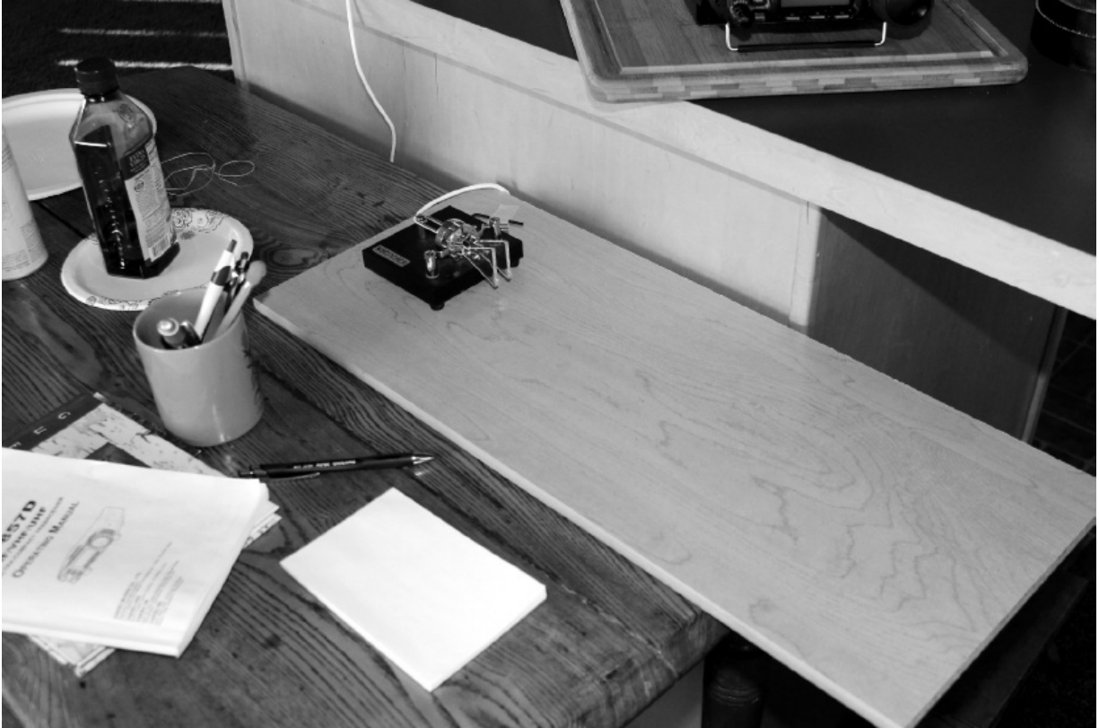
FIGURE 6-11 A Bencher CW keyer paddle, glued down with contact cement to a wooden board for portable operation.
