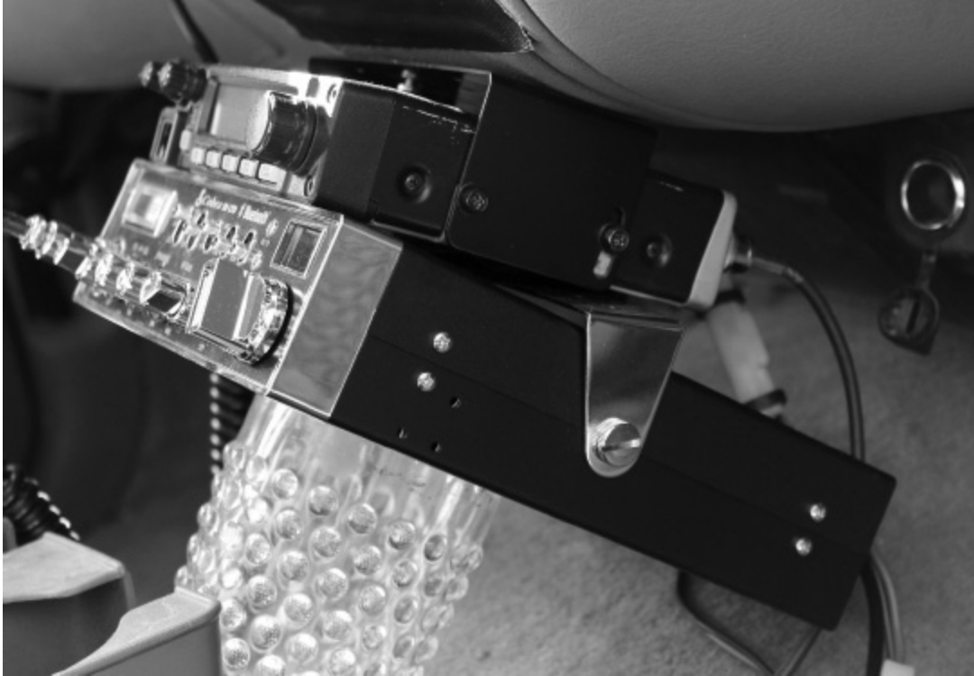
FIGURE 1-4 Two-way radios mounted under the dashboard of my vehicle. An amateur mobile transceiver rests on top, and a CB mobile transceiver sits underneath it. A plastic cup, wedged underneath the CB radio, keeps both units from wobbling.
