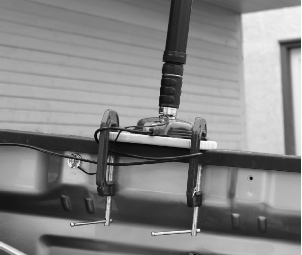
FIGURE 6-15 The base mount that I devised for the ATAS. Note the ground wire going from the base of the ATAS to a screw in the truck bed.
