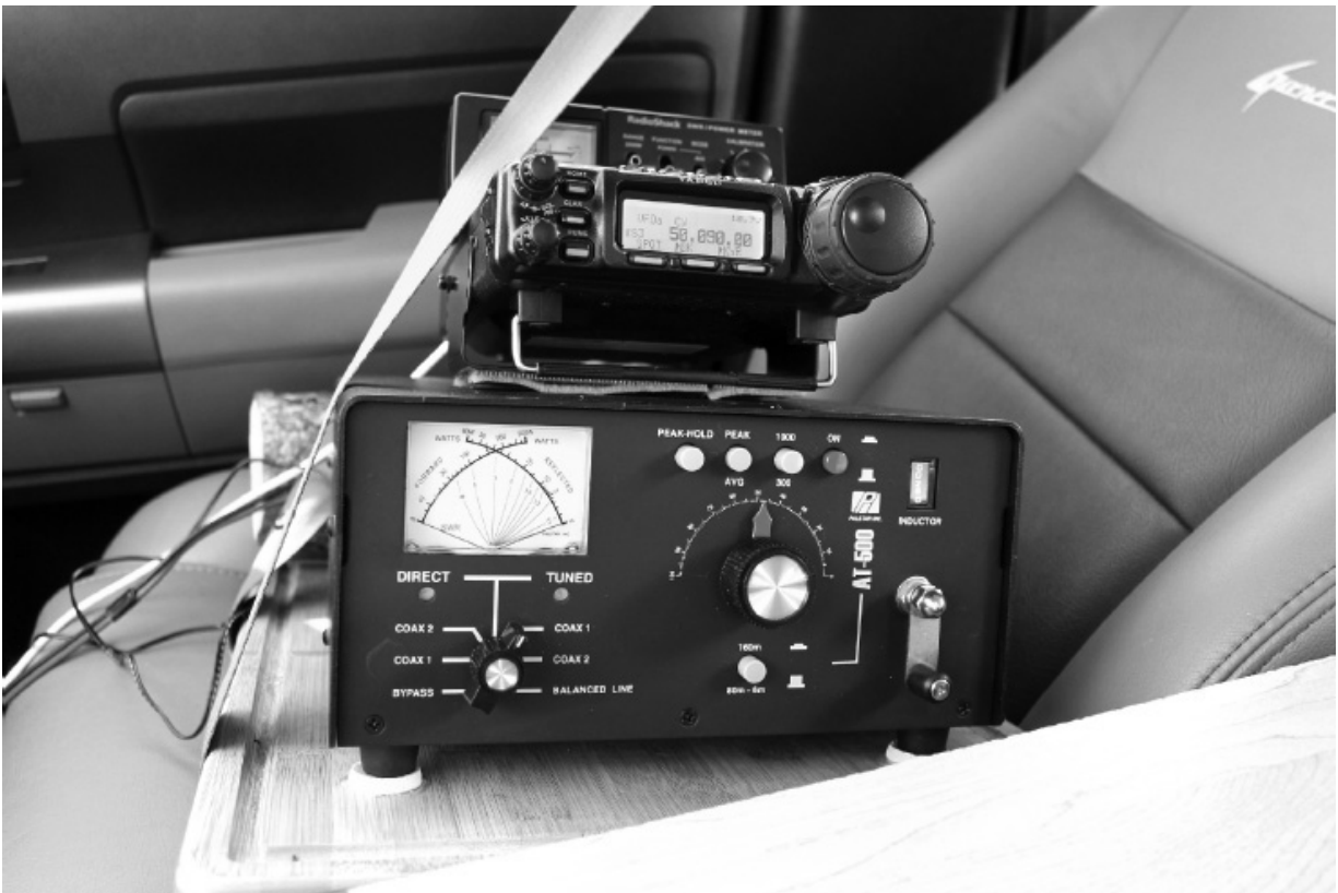
FIGURE 6-6 A transmatch in a mobile installation for increasing antenna bandwidth and operating on bands at frequencies far different than that of the antenna's design band. In my arrangement, the radio sits on top of the transmatch.
