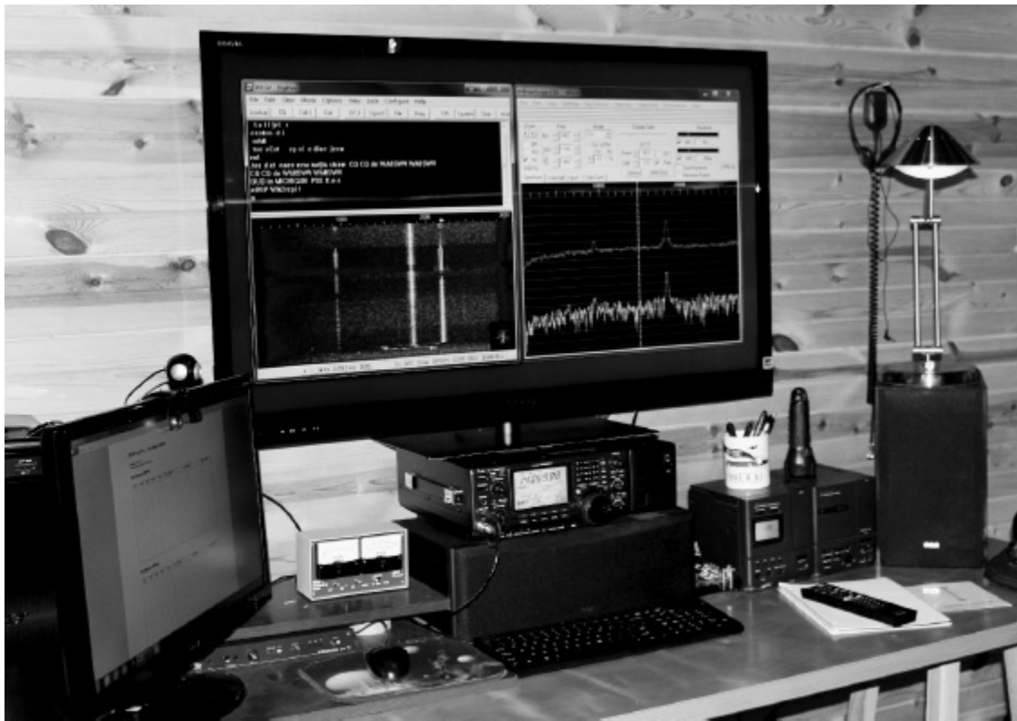
FIGURE 1-1 My ham radio station includes a transceiver, an Internet-ready computer, an interface for digital communications, a power output and antenna testing meter, an audio amplifier with four speakers (one shown here, at extreme right) and two displays, one of which is a 46-inch high-definition television set.
